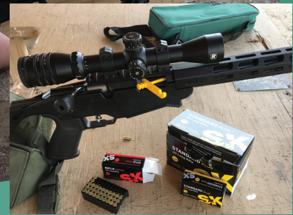
One of the RPRs with a Redfield tactical .22 BDC reticle scope. Sight it in for 50 yards and it has marks for 75, 100, 125, and 150. This is the first time we used SK ammunition, both standard .22LR and match. The match was slightly better resulting in outstanding and consistent groups.
